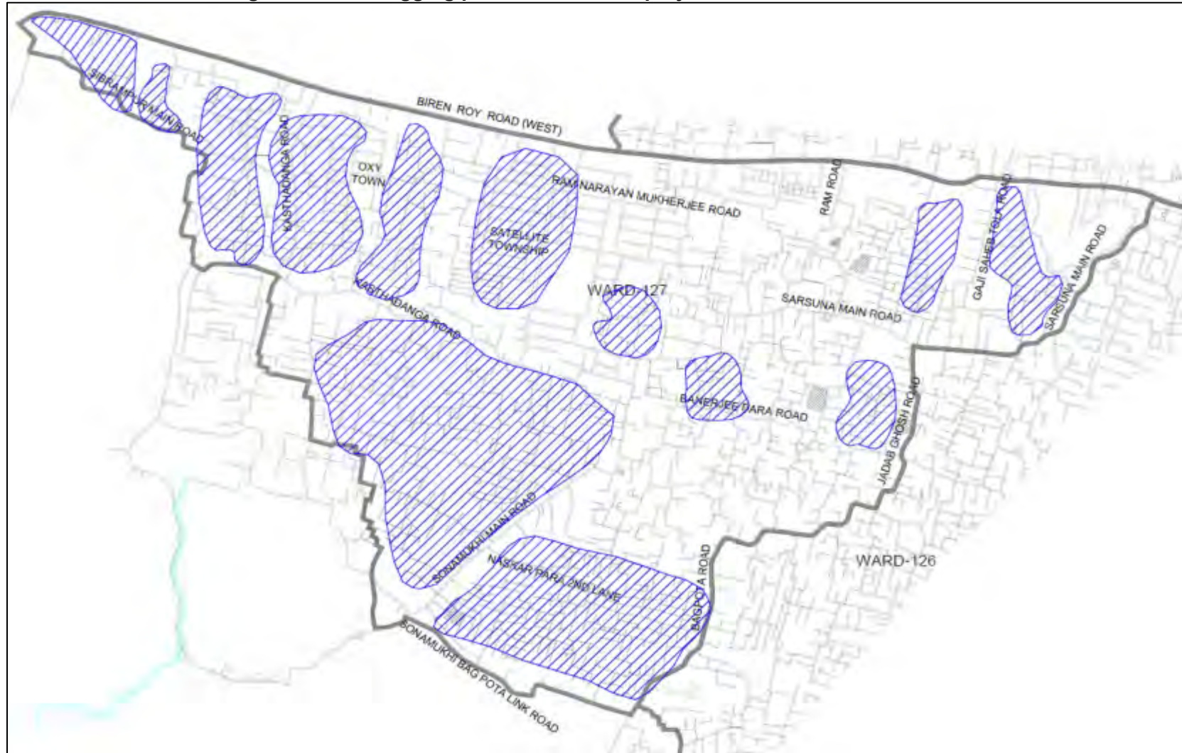
Figure 6: Waterlogging pockets in the subproject area of SD 08 and SD 09
