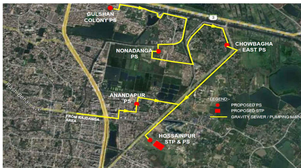
Figure 3: Transmission of DWF to proposed Hossainpur STP
