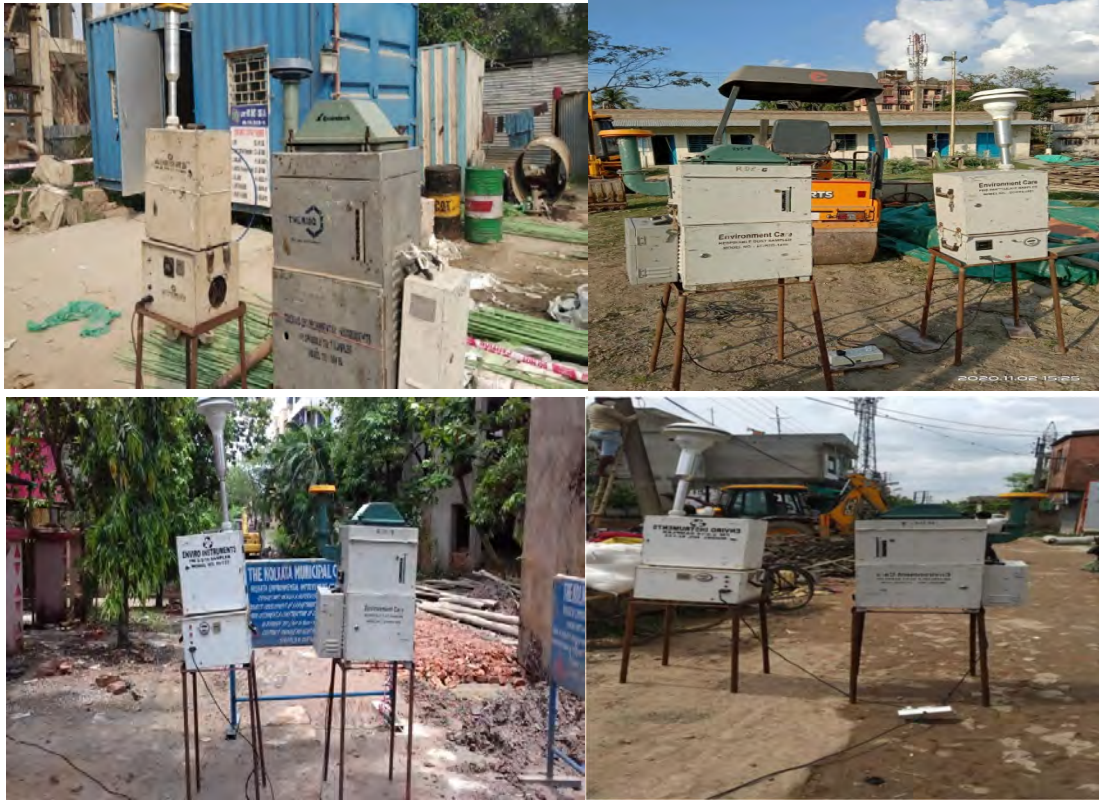
Ambient Air quality monitoring at project sites
